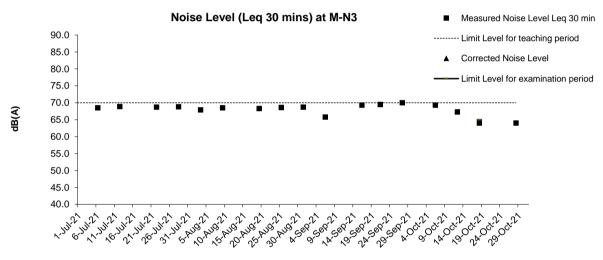
Remark: Corrected Noise Level = Measured Noise Level - Baseline Noise Level (i.e. 67.7 dB(A))
